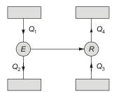
In the figure shown above, E is the heat engine with efficiency of 0.4 and R is the refrigerator. If  $Q_2 + Q_4 = 3Q_1$ , the COP of the refrigerator will be
